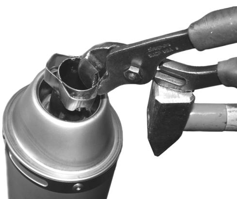
3) Pull the bushing out and loosen the allen screw that is under it.
