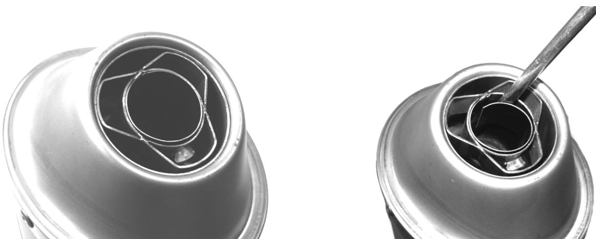
1) Inside the dB eater is a thin bushing securing the allen bolt.
